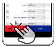
Tap **Stop** to end the recording. VuSitu displays a summary of the live readings data.
