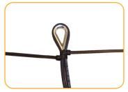
Place the second zip tie directly below the first and tighten.
