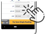
From the Live Readings screen, tap the settings wheel next to the field that contains the measurement value.
