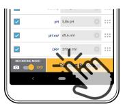
Tap **Start Recording**. The instrument takes a reading every two seconds.
