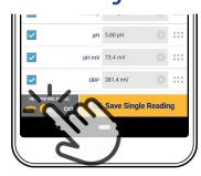
Tap the button on the bottom left to switch from snapshot mode to live readings mode.
