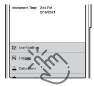
Pair VuSitu with the instrument. Select **Logging** from the Connected Instrument screen.
