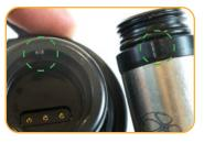
Invert the instrument. Align the notch on the instrument with the tab on the rim Rugged TROLL Cable. This will ensure that the pins are aligned to enable communication.
