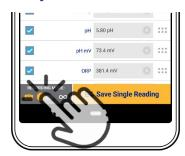
Tap the button on the bottom left to toggle between snapshot and live readings modes.
