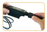
Attach the Rugged TROLL Connect the Com to the Rugged TROLL 200 cable via snap-on connection to the uphole end of the cable.
