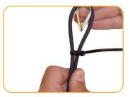
Place the metal loop inside the cable loop.
